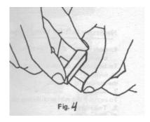
While pressing blocks slightly together, turn them through 90°. Slide the blocks from side to side each other under light pressure until wringing begins to take place, as shown in the figure.
